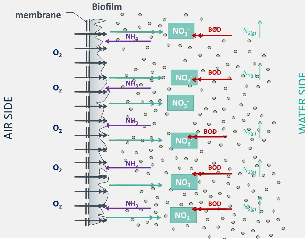
**Autotrophic** biofilm develops at low BOD conditions, nitrifies ammonia using oxygen from the membrane
