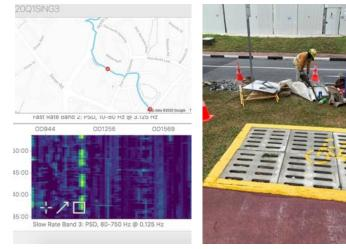
DigitalAsset Deployment in Singapore: Detection 4 March 2020 – Jackhammer verified. (Cable depth 1.2m; Activity lateral offset to cable/water pipe: 23m)
