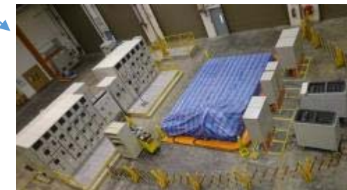
500kW Motor Testbed – Flexible platform for testing of motors, generators and electric drives
