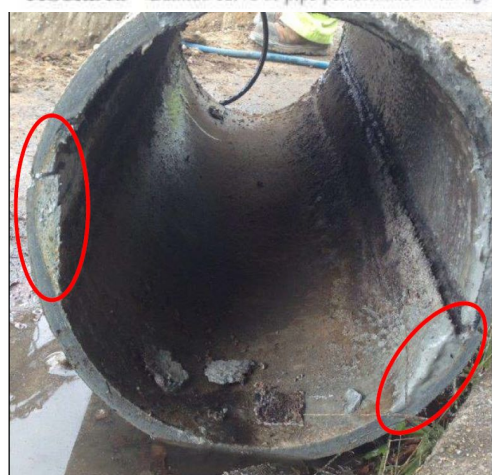
Delaminated areas of AC pipe
